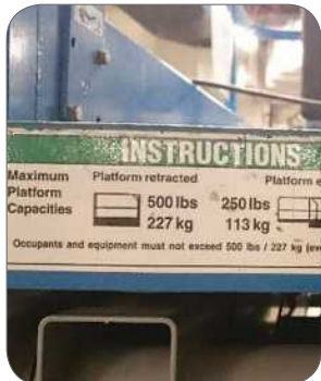
Figure 10: A safe working load label.
