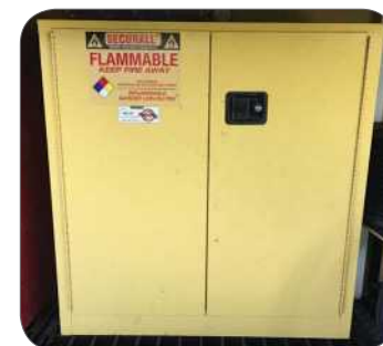
Figure 21: Storage cabinet with label and lock.
