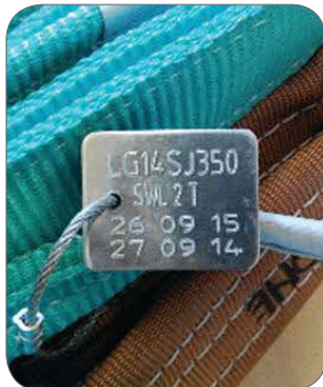
Figure 11: A tag with safe working load, inspection date and expiry information.
