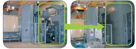
Figure 4: Enclosure of noise generating chamber blast pot.
