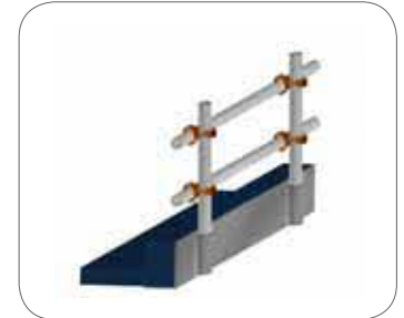
Figure 30: Example of edge protection off the structure.
