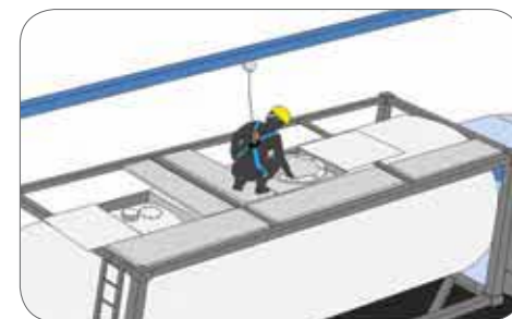
Figure 36: Drive-in anchorage and lifeline structural system.
