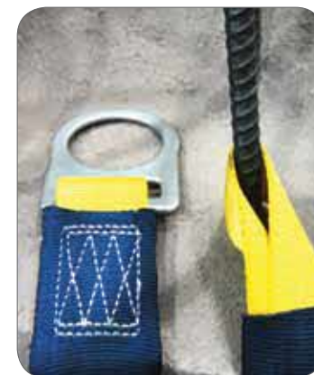
Figure 41: Example of a strap anchor.
