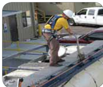
Figure 38: A proprietary TRAM system by Standfast Corp.
