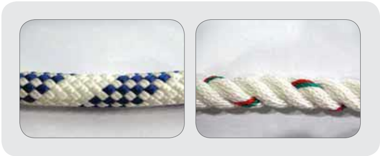
Figure 10: Examples showing a kernmantel (left) and hawser-laid lifeline.
