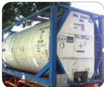
Figure 32: Example of a tank container.
