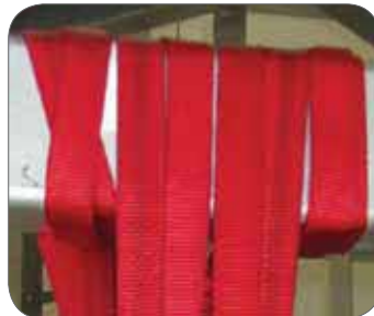
Figure 7: Excessive looping of an anchor sling should be avoided (unless otherwise stated in manufacturer's manual).
