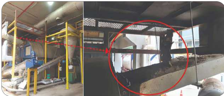
Figure 16: The force from the dust explosion spread to the relief vent which blasted open.
