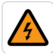
W015 Warning: Electrical hazard
