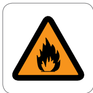
W012 Warning: Flammable material
