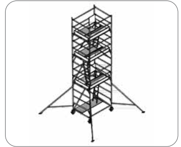
Figure 22: A mobile scaffold with access ladder, opening and other features to provide a hazard-free working platform.
