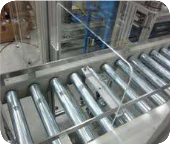
Figure 18: Engineering control: use of a mechanised system to transport objects.
