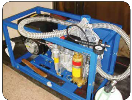
Figure 18: Typical HP air compressor.
