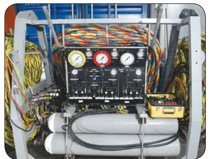
Figure 14: Typical frame-mounted SRP with dive control panel and communication box.
