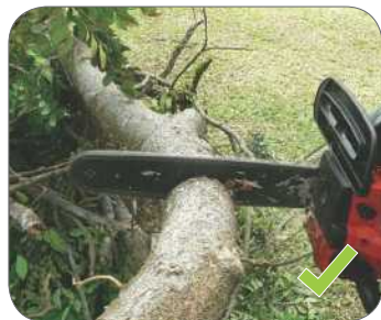
Figure 38: To avoid kickback, use the base of the blade when cutting logs.
