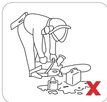
Figure 42: Do not start the saw at the place of refuelling.
