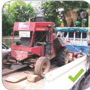
Figure 118: Use tie-down or other means to secure the equipment during transportation.
