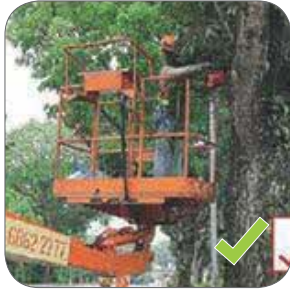
Figure 46: Stay within the work platform at all times and do not overstretch to cut the branches. Hook the safety harness to a designated anchorage point.
