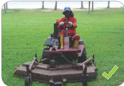
Figure 24: Safety guard should be in place before operating the ride-on mower.
