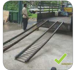
Figure 119: Use appropriately designed ramps for unloading and loading equipment.
