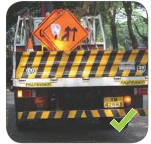
Figure 113: Mount blinking beacon lights on top and rear of vehicles.
