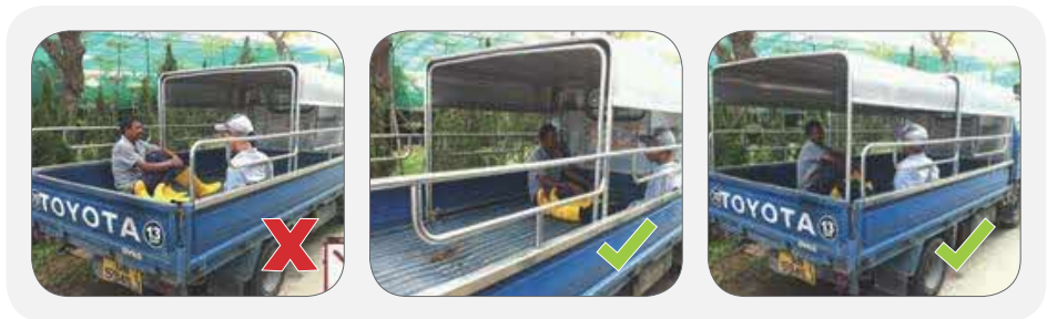
Figure 116: Ensure that there is sufficient space for each worker and the canopy cover is available.
