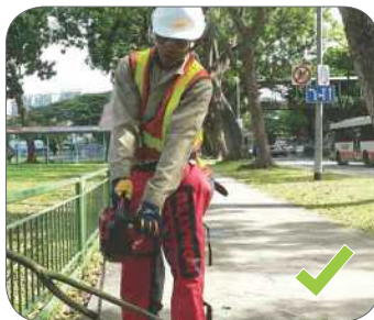
Figure 39: Do operate a chainsaw with both hands.
