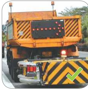
Figure 112: Use Truck Mounted Attenuator (TMA) when working on expressways and roads with speed limit above 70km/h.
