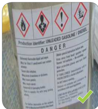
Figure 91: Labelled chemical container.
