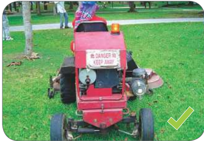
Figure 23: Place warning sign and mount blinking lights on the mower.
