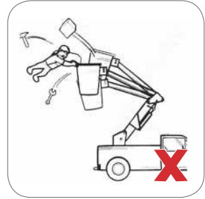
Figure 48: Do not drive an MEWP with the worker in the bucket.
