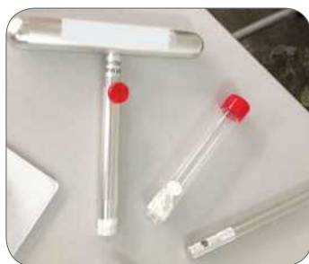
Figure 17: A core sampler.
