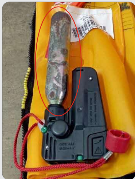
Figure 6: Corroded gas cartridges
