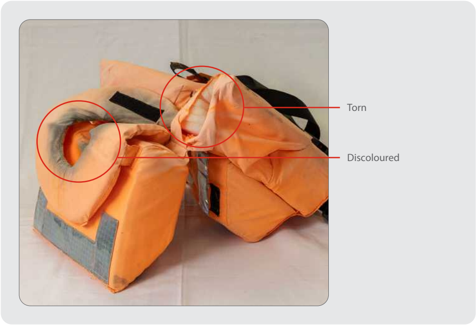
Figure 10: Discoloured and torn foam life jacket
