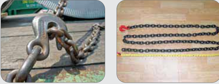
Figure 22: Steel chains with a grab hook attached on one end.
