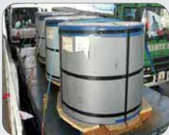
Figure 50: Coiled sheet metal loaded on pallets and lashed.
