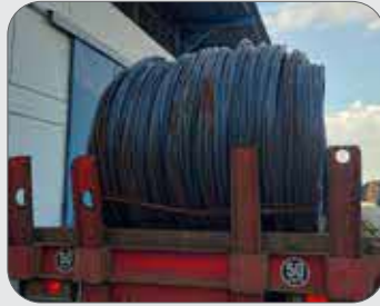
Figure 48: Wire coils lashed and blocked with a metal bracket at the rear.
