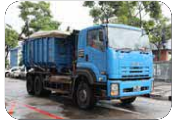
Figure 46: Skip container transporting construction debris.
