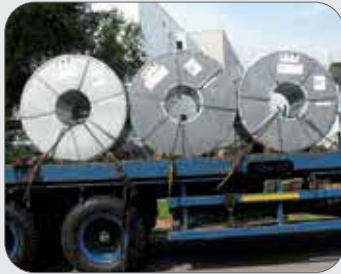
Figure 49: Sheet metal rolls chocked with dunnage (left) loaded within metal brackets (right).
