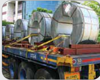
Figure 49: Sheet metal rolls chocked with dunnage (left) loaded within metal brackets (right).
