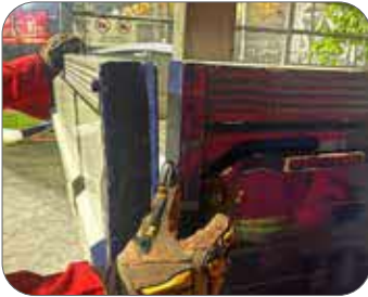
Figure 9: Example of a pinch point hazard.
