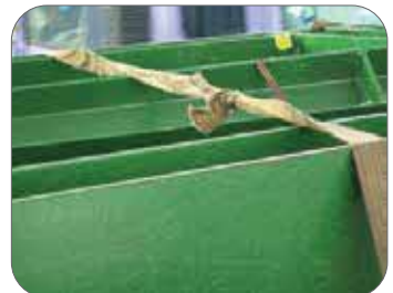
Figure 24: Bad practice of tying two lashing belts.
