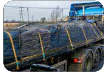
Figure 25: Tying down cargo on truck bed with load securing net.
