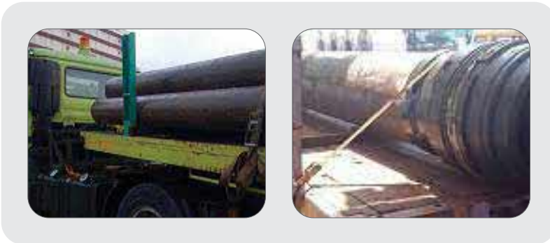
Figure 53: Steel pipes loaded against stanchion and lashed to loading platform.
