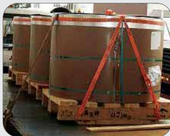
Figure 50: Coiled sheet metal loaded on pallets and lashed.
