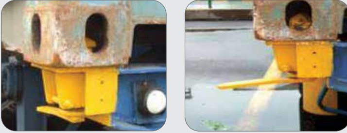
Figure 32: Twistlocks in locked and unlocked positions.
