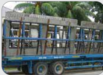
Figure 58: Trailers mounted with steel frames for transporting precast concrete.
