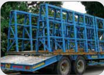
Figure 58: Trailers mounted with steel frames for transporting precast concrete.
