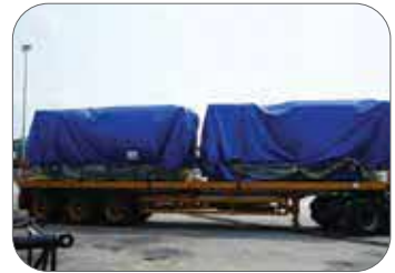
Figure 26: Cargo covered with sheets for weather protection.
