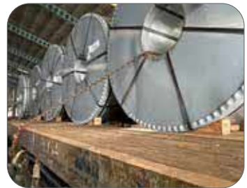
Figure 36: Cylindrical cargo being wedged.
