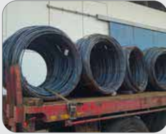
Figure 48: Wire coils lashed and blocked with a metal bracket at the rear.
