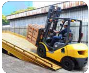
Figure 4: Example of a ramp operation.
