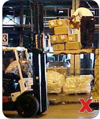
Figure 2: Unauthorised use of forklift to elevate personnel.
