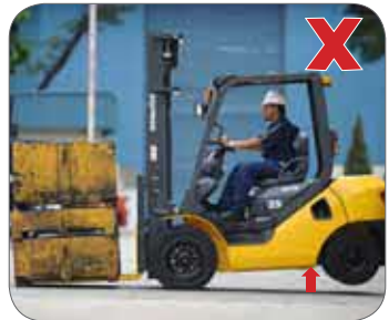
Figure 3: Example of an overloaded forklift.
