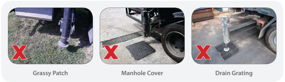
Figure 3: Locations where outriggers should NOT rest on
