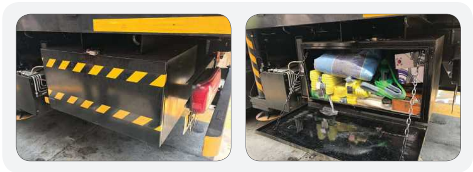
Figure 12: Example of proper storage area for lifting gears
