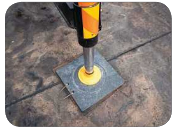
Figure 5: An outrigger sitting on a stabiliser pad
