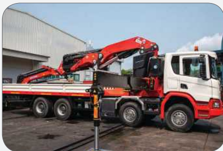
Crane boom rested on deck
