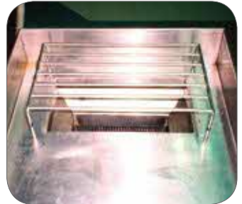
Figure 30: After the accident, shaft cutters were guarded to prevent future mishaps.
