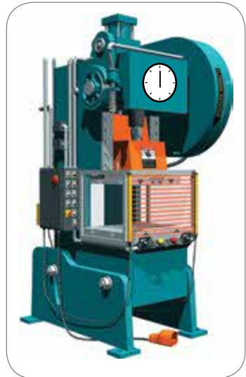
Figure 19: Machine equipped with a safety light (picture courtesy of Omron STI).
