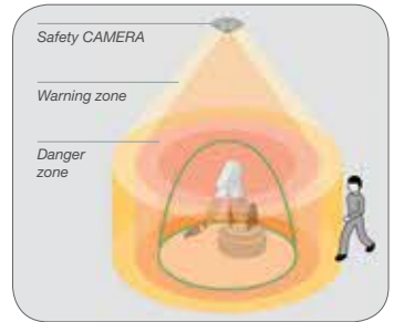
Figure 21: Example of a safety camera system.
