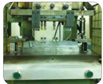
Figure 22: Example of a two-handed control device on a power press.
