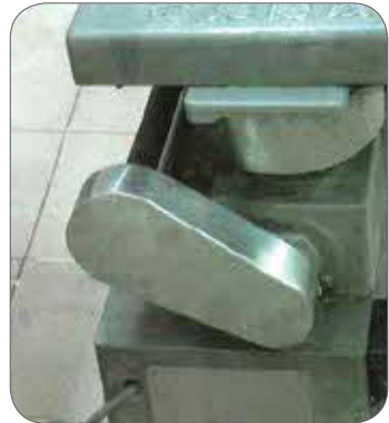
Figure 14: Fixed guard to prevent access to danger zone from all directions.
