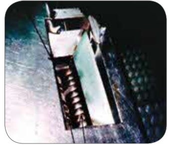
Figure 29: Unguarded rotating shaft cutters that pulled the operator's hand in.
