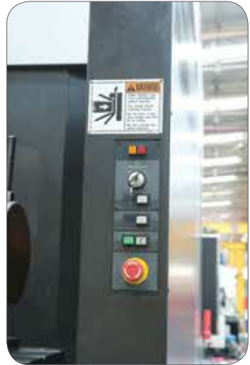
Figure 23: Example of an emergency stop device.
