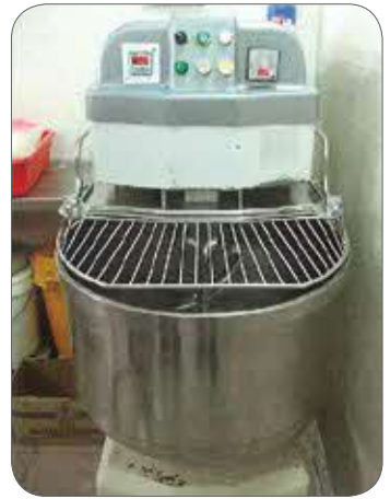
Figure 17: Flour mixer installed with interlocking guard.
