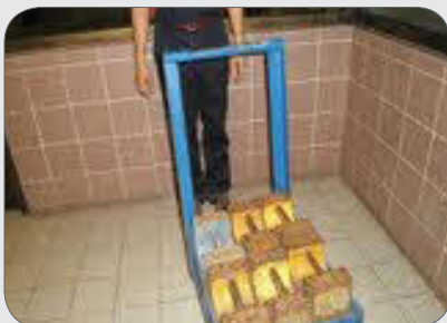
Figure 44: Loading/unloading – test weight (using lorry crane / movable platform / forklift / trolley)
