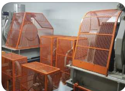
Figure 72: An example of safety guards provided for moving parts
