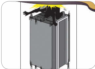
Figure 10: Being trapped between an ascending lift car and the soffit of the lift shaft
