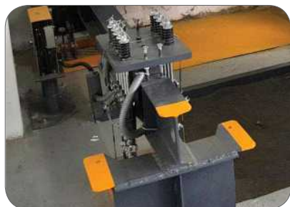
Figure 79: Round off the edges or corners of machine beams and marking of sharp edges
