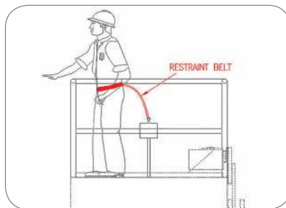
Figure 98: Hooking up of restraint belt
