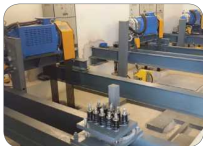
Figure 71: An example of safety guards provided for moving parts
