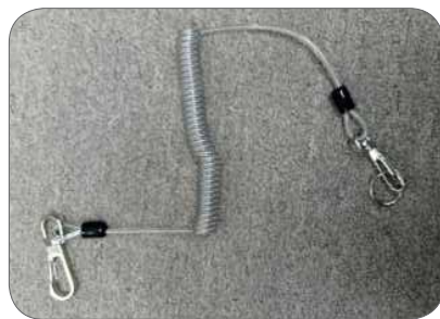
Figure 107: Tool lanyard/tie down cord to prevent hand tools from dropping while working on car top without entanglement hazard with any moving part
