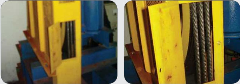
Figure 68: An example of pulley guards with a viewing window for rope inspection
