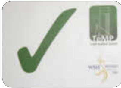
Figure 109: Check "Safe to use tag" is valid
