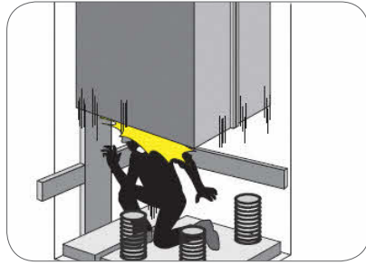
Figure 13: Being trapped between a descending lift car and the bottom of the lift pit
