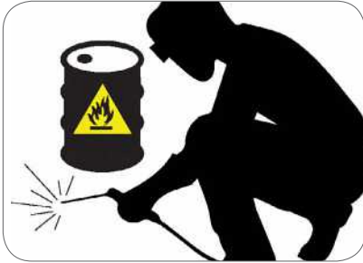
Figure 47: Welding operations with the presence of flammable substances in the vicinity
