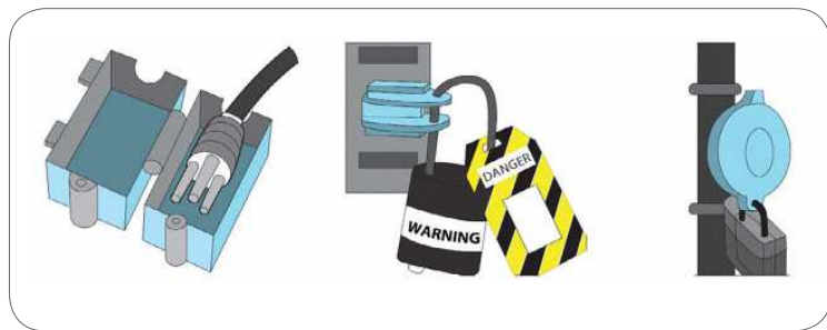
Figure 78: Examples of using lockout and tagout to isolate the source of electrical energy in the machine room
