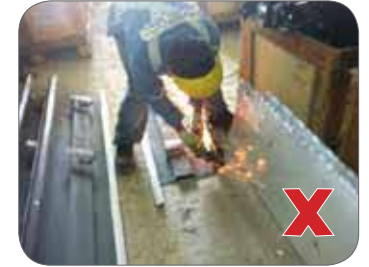
Figure 38: Fire hazard presented by welding, grinding, plasma cutting or gas cutting (above).
