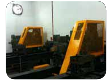
Figure 49: Example of pulley guards with a viewing window for rope inspection.
