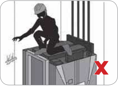
Figure 32: Hand tools falling from lift car top down to hoist way.
