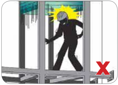
Figure 5: Being trapped between a descending lift car and counterweight inside the hoist way.
